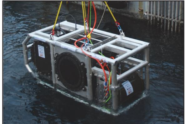
Figure 1: The GDAPS Marine Vibrator Integrated Projector Node (MVIPN) undergoing performance verification testing at NUWC Seneca Lake Sonar Test Facility in Dresden NY
