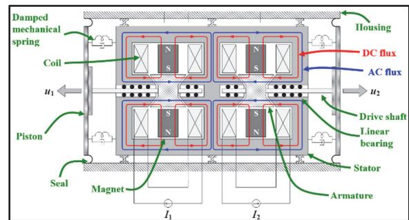
Figure 2: GDAPS marine vibrator transducer schematic
