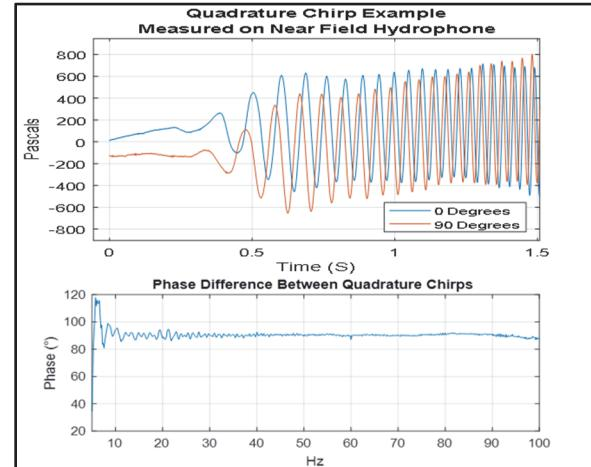
Figure 6: The 5Hz-100Hz linearly swept sine waveform is transmitted with 0 and 90 degree phase shifts
