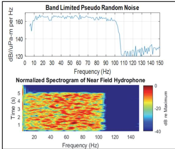
Figure 5: Measured spectrum and spectrogram of a 5 second long pseudo random noise transmission
