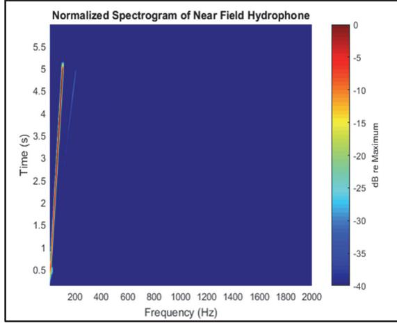
Figure 4: Hydrophone data spectrogram of a 5 second long, linearly swept 5Hz-100Hz seismic sweep on 40dB scale
