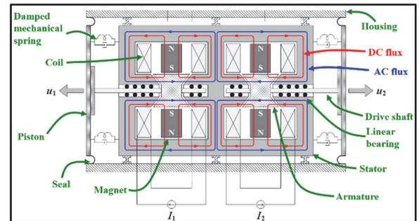
Figure 2: GDAPS marine vibrator transducer schematic
