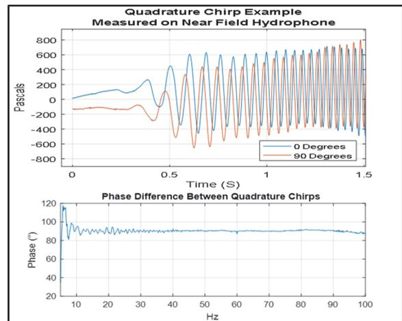
Figure 6: The 5Hz-100Hz linearly swept sine waveform is transmitted with 0 and 90 degree phase shifts
