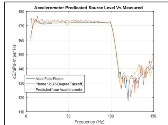
Figure 3: Comparison of the accelerometer prediction of source level and measured source level using calibrated hydrophones.
